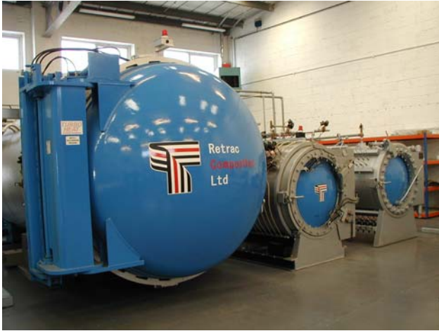
Autoclaves at RCL for curing thermoset polymer matrix composite components
